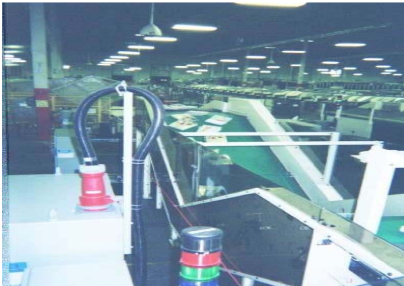
Illustration 1. We observed Standard A mail bundles breaking apart on the APPS induction conveyor system waterfall.
