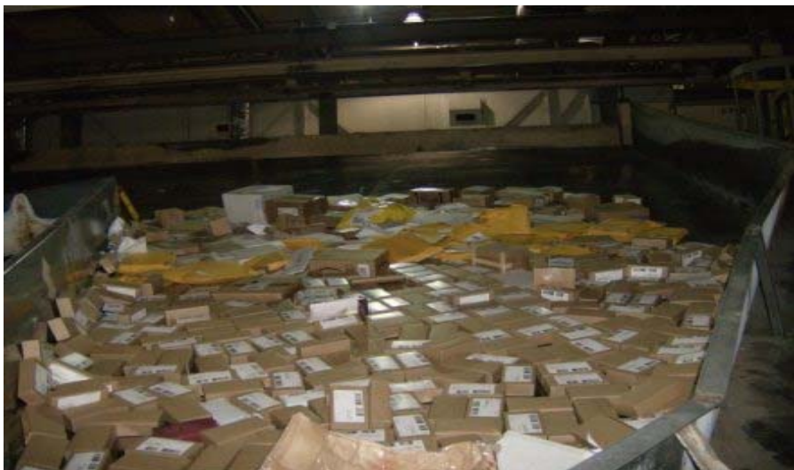
Illustration 5. Mail directed to keyers rather than SSIUs. Small parcels with an SSIU readable barcode were processed by parcel sorter keyers rather than by the more efficient SSIU, resulting in the use of unnecessary workhours. (April 25, 2006.)
