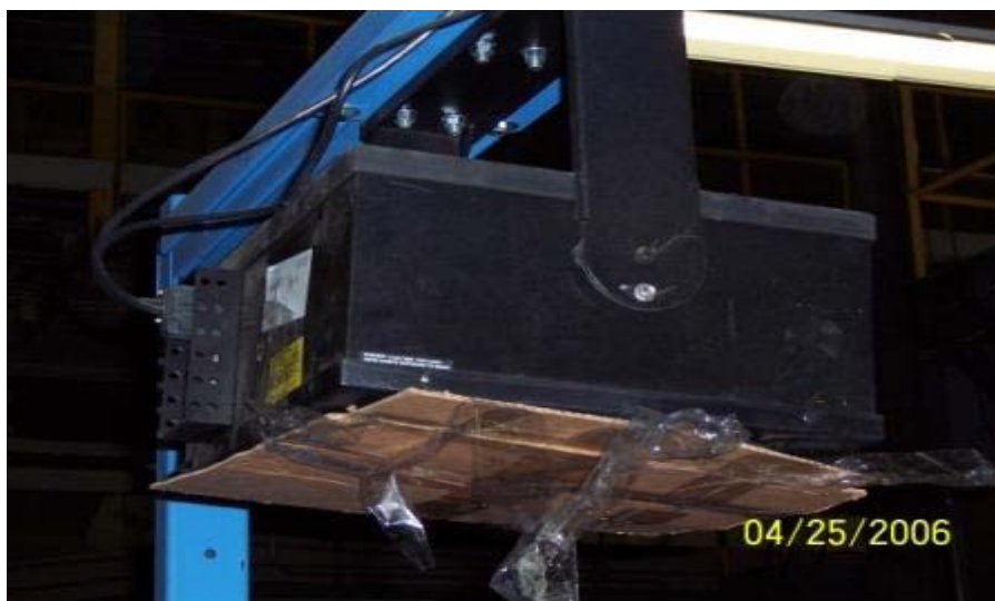
Illustration 7. Scanner disabled on Universal Sorter. The Universal Sorter barcode scanner was disabled, requiring the use of keyers. This resulted in lower productivity. (April 25, 2006.)
