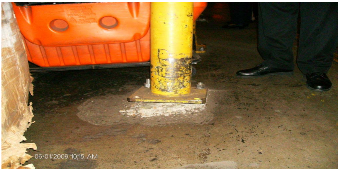
Illustration 8: A safety post with bolts sheared off from impact from a PIV.
