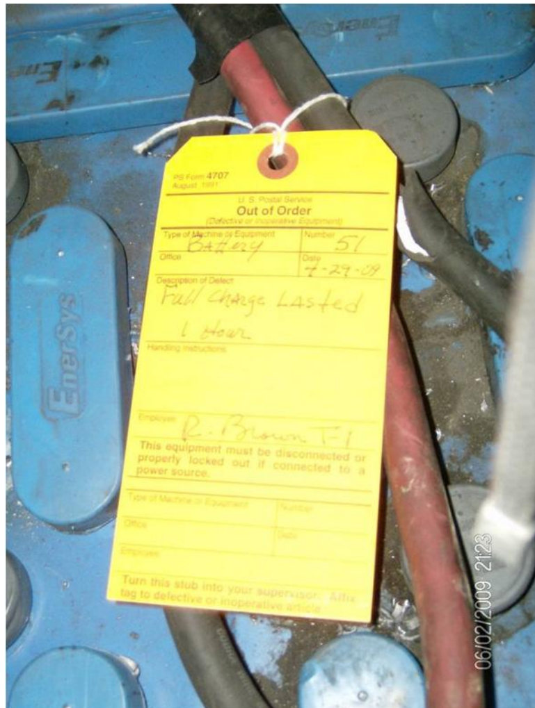
Illustration 12. Example of tag on a battery. It says "Full charge lasted 1 hour."
