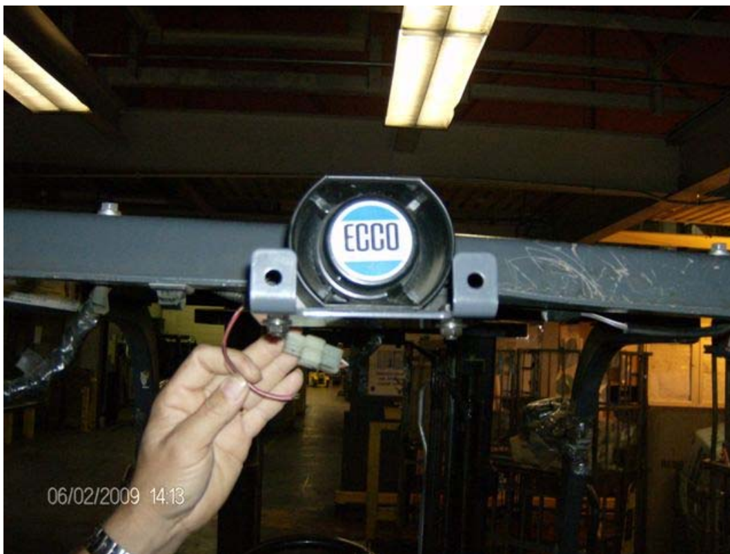
Illustration 9: The warning horn on vehicle did not work because the wire had been cut.
