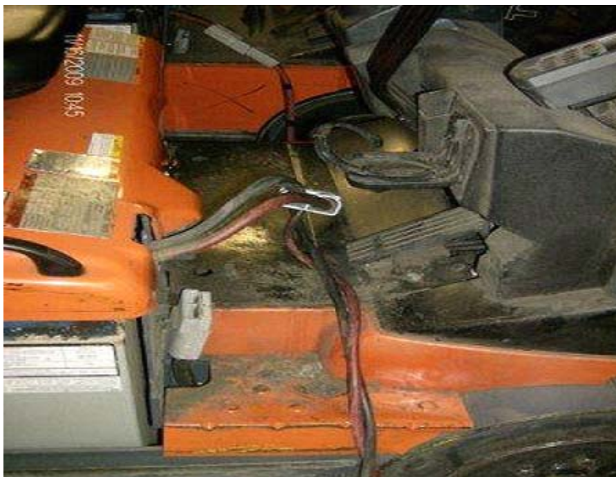
Illustration 2: An employee charged a forklift vehicle battery at the Indianapolis P&DC without removing it from the vehicle on 11/16/09.
