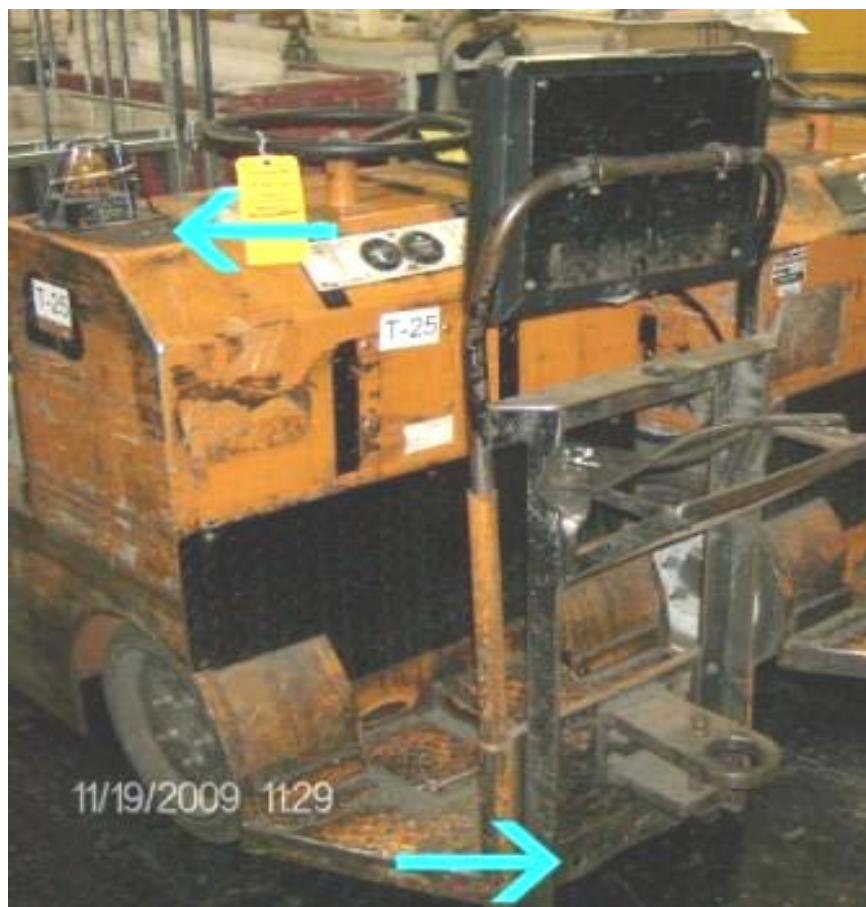
Illustration 5: Tow vehicle without a PIVMS VAC or tow sensor at the Indianapolis P&DC on 11/19/2009 at 11:29 a.m. The top arrow shows where the VAC was originally mounted. The bottom arrow shows where the tow sensor was originally mounted.
