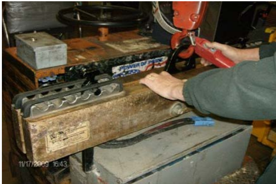
Illustration 1: A battery being removed from a tow vehicle with a hoist on 11/17/09 at the Indianapolis P&DC. Employees discharged tow vehicle batteries and then removed them from the vehicles and recharged them.
