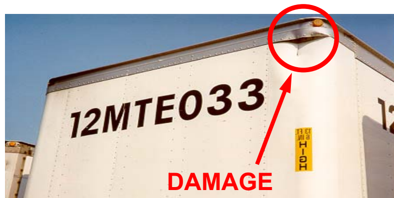
Figure 7 – Trailer damage at a mail transport equipment service center.
