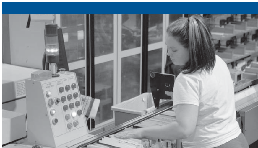
The Postal Service primarily uses two types of equipment to sort letter mail into walk sequence. There are the high-speed delivery barcode sorters (DBCS) machines in the plants and the less efficient carrier sequence barcode sorter (CSBCS) machines in the associate offices.
