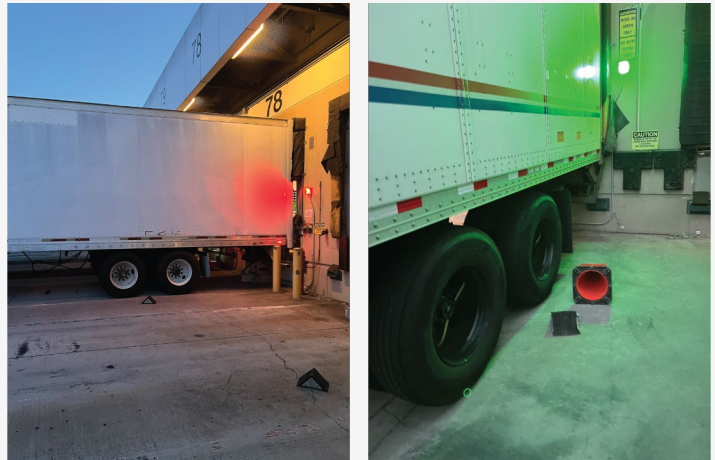
Figure 4. Trailers Without Wheel Chocks
